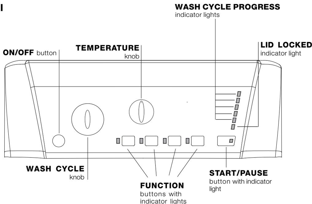
**ON/OFF** button: switches the washing machine on and off.
